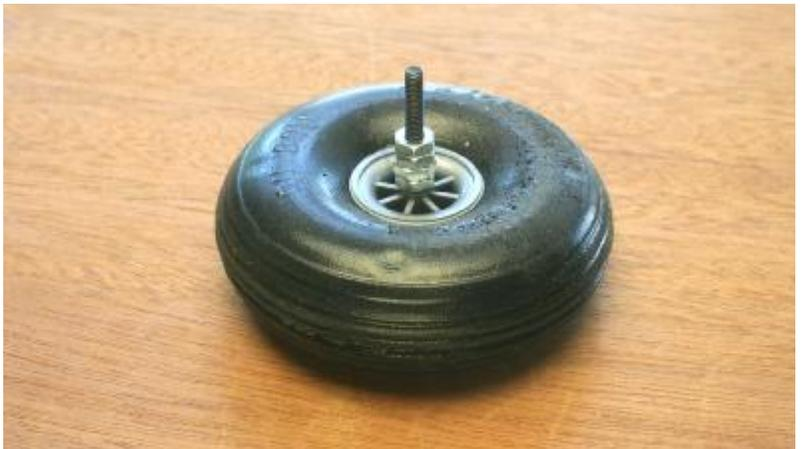
3...Insert the axle into the landing gear and secure with a nut. Use a thread locking compound on this nut.
