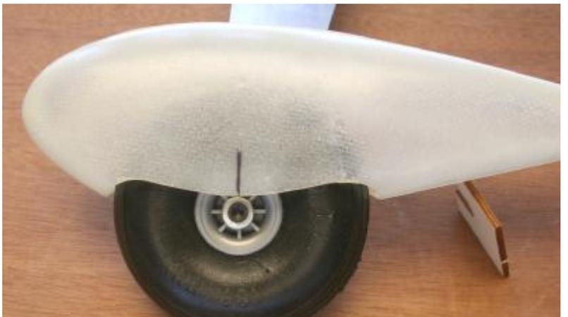
5...Place part LG on the inside of the wheel pant as shown. The inboard corners on the bottom should be flush with the wheel pant. The outboard corners of LG should extend below the edge of the wheel pant an equal amount. Glue part LG to the inside of the wheel pant with thick C/A glue.
