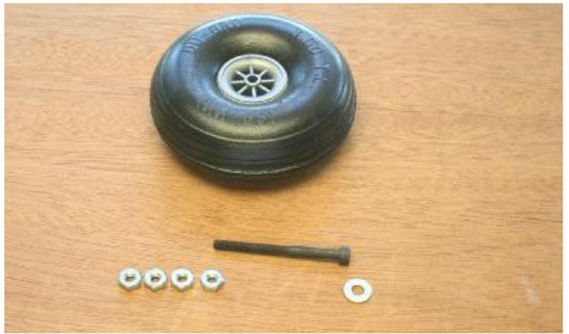
2...Place a washer on the axle screws. Insert the axle screws into the wheels. Install one nut on the axle and screw it down to the wheel. Back the nut off 1 turn to allow about 1/32" side play in the wheel. Now install a second nut to lock the first one in place. Now install a third and fourth nut as a spacer. Use a thread locking compound on these nuts.
