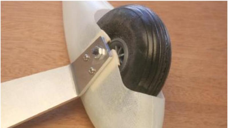
11...Repeat to install the wheel pant on the opposite side. Make sure the wheel pants are aligned with each other.
