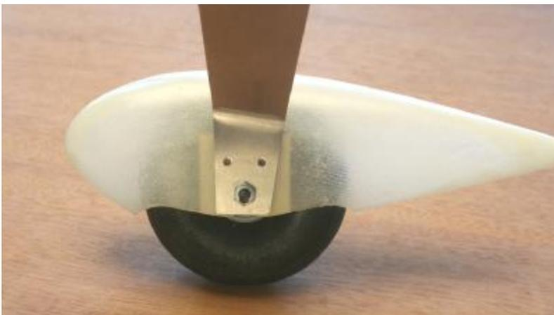
8...Drill the screw holes in the wheel pant with a 5/32" drill bit.
