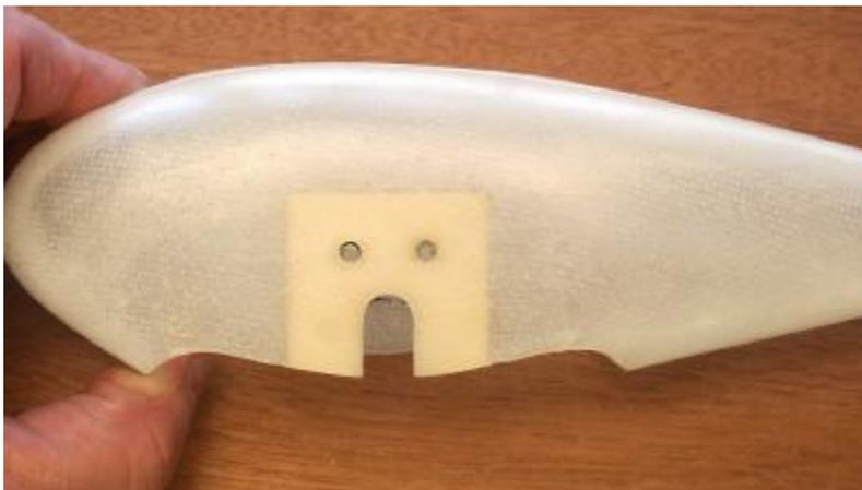
9...Tightly press the two 4-40 blind nuts into the holes in part LG. Secure them with a small drop of C/A glue.
